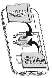
Take care not to scratch or bend the contacts on the SIM card. Should you need, but have problem to remove/replace the SIM card, use adhesive tape on the exposed part of the SIM card to pull it out.
