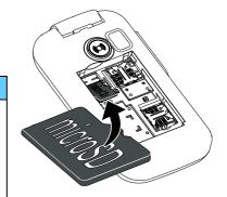
**Note!** Since the SIM card holder and the memory card holder are located beneath the battery you need to turn off the phone to insert or remove the cards.
