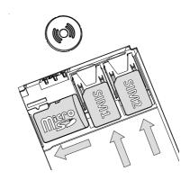
Take care not to scratch or bend the contacts on the SIM card. Should you need, but have problem to remove/replace the SIM card, use adhesive tape on the exposed part of the SIM card to pull it out.
