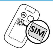
This device accepts a **micro-SIM card** or **3FF**. Use of incompatible SIM cards may damage the card or the device, and may corrupt data stored on the card.
