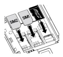
Take care not to scratch or bend the contacts on the SIM card. Should you need, but have problem to remove/replace the SIM card, use adhesive tape on the exposed part of the SIM card to pull it out.
