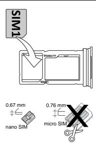
You may optionally place a memory card in the tray. Make sure that the memory card's contacts are facing downwards and matching the slot tray. Compatible card type: microSD, microSDHC, microSDXC, max 1024 GB.
