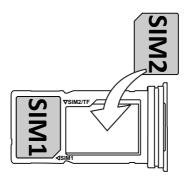
• Insert the SIM card tray back into its slot. See *External memory*, p.64 for additional info.
