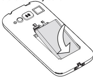
Insert the battery by sliding it into the battery compartment with the contacts facing downwards to the right. Replace the battery cover.
