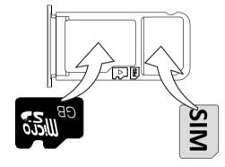
Make sure that the SIM card's contacts are facing downwards and that the cut off corner is down, as shown. Take care not to scratch or bend the contacts on the SIM card.
