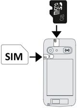
2. You may also optionally insert a memory card. Make sure that the memory card's contacts are facing downwards, as shown. To remove the memory card: find the small ridge on the exposed end of the memory card. Put your fingernail into the ridge and gently pull the memory card out. Compatible card type: MicroSD, MicroSDHC, MicroSDXC
