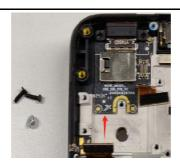
3. Carefully wiggle and pull the **USB PCB** to remove it.
