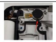
5. Insert the **Prying lever** into the groove next to the **Speaker** and gently pry it up.
