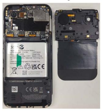
4. Remove the **LED light board foam** from the **Rear housing ASSY**.
