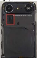
2. Remove the Screw2 bracket marked red.
