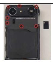
3. Use a Prying lever or a Plectrum to pry off the Rear housing ASSY.
