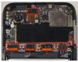
2. Remove the Screw3 PCBA.
