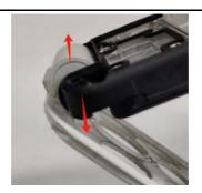
3. Separate the Front housing ASSY and the Hinge Flip bottom ASSY.
