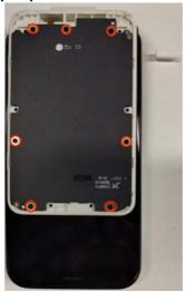
3. Carefully turn the **PCBA ASSY** around to not damage the **FPC**, the disconnect the **FPC**.
