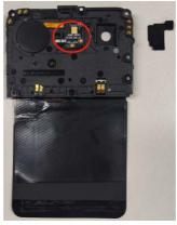
6. Use a pen to push out the **rear camera lens** from the back side of the **Rear housing ASSY**.
