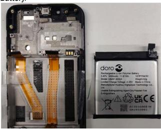
4. Remove the remaining protective film to separate the material from the **Battery**.
