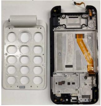
4. Use the **Screwdriver** to push out the **hinge**.
