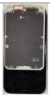
2. Remove the Screw4 flip top bottom cover.
