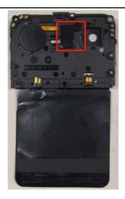
5. Remove the Flash PCB from the Rear housing ASSY.
