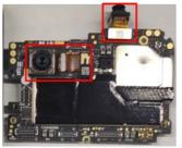
5. Remove the Rubber sleeve front camera from the Front camera 5M.
