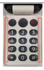
2. Insert the **Plectrum** between the **Hinge Flip bottom ASSY** and the **Flip decorative part** to pry up the **Flip decorative part**.
