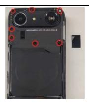
3. Use a Prying lever or a Plectrum to pry off the Rear housing ASSY.
