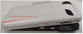
4. Once fully loosened, carefully lift off the Battery cover ASSY.
