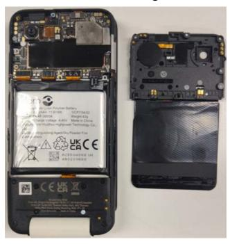
4. Remove the **LED light board foam** from the **Rear housing ASSY**.
