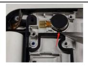
5. Remove the **Sealing silicone C hinge** using **Tweezers**.
