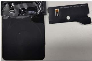
10. Disconnect the **FPC** on the **NFC antenna** by peeling it off using **Tweezers** or a **Prying lever**.
