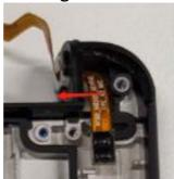
2. Separate the the **Sealing silicone A hinge** from the **Hinge FPC**.
