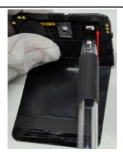
7. Disconnect the two **FPC** on the **NFC antenna** by peeling them off using **Tweezers** or a **Prying lever**.
