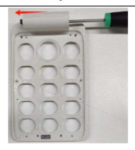
5. Separate the **Hinge Flip bottom ASSY** and the **hinge**.
