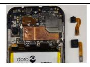
6. Remove the Rubber sleeve front camera from the Front camera 5M. Remove the Rubber sleeve wide angle camera from the Wide angle camera 5M.
