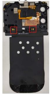
4. Remove the **Flash board cooling silicone** [**H695-0330-NQ0**]. Then remove the **Receiver ground conductive foam** [**H186-0668-UW0**].
