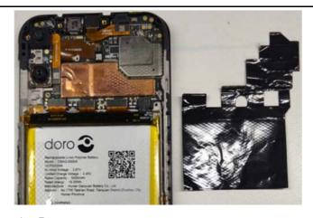
2. Disconnect the Battery connector.
