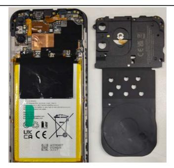
3. Disconnect the two FPC on the **NFC antenna Charging coil** by peeling them off using **Tweezers** or a **Prying lever**.
