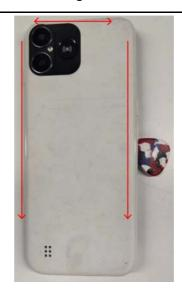
3. Once the top and side edges are loosened, firmly push the **Battery Cover ASSY** toward the bottom of the device.
