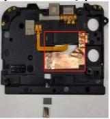
6. Remove the Flash PCB from the Rear housing ASSY.
