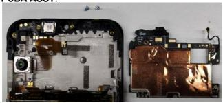
4. Remove the **Sensor rubber sleeve** and disconnect and remove the **Pilot lamp board RF cable**.
