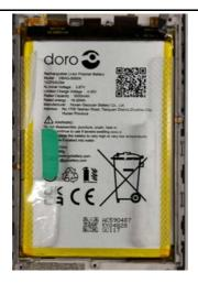
2. Firmly pull the remaining plastic strip to lift the **Battery** out of the battery compartment.
