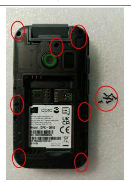
2. Insert the **Plectrum** at the bottom of the device and gently pry open the **Lower housing assembly**. Start at the bottom, continue along the sides, and work your way around.
