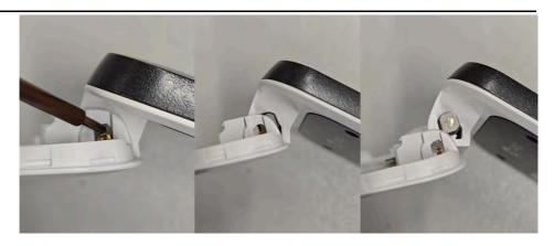
2. Separate the Clamshell assembly and the C-cover.
