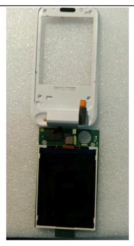
2. Disconnect the **FPC\_LINK\_SF28A\_GF28A1\_6L\_HOLE\_V01A** using **Tweezers**.
