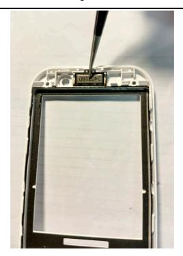
2. Remove the **Motor** from the **Clamshell up assembly**.
