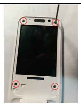
3. Carefully separate the **Clamshell up assembly** from the **Clamshell assembly** along the edge with a **Plectrum**.
