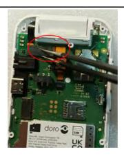
2. Grip the edge of the PCBA assembly HW3011 and lift it gently.
