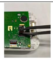
3. Lift the Camera using Tweezers.
