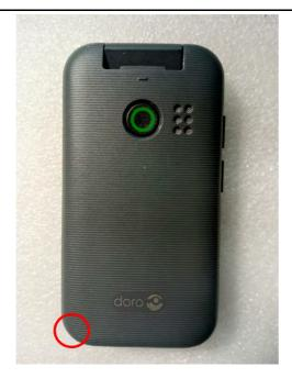
3. Insert a **Plectrum** into the notch and gently slide it along the edges to lift the **Battery cover**.
