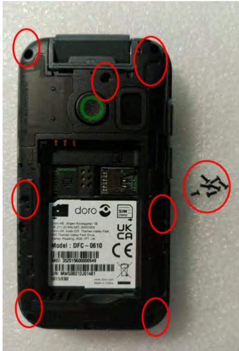
2. Insert the **Plectrum** at the bottom of the device and gently pry open the **Lower housing assembly** . Start at the bottom, continue along the sides, and work your way around.
