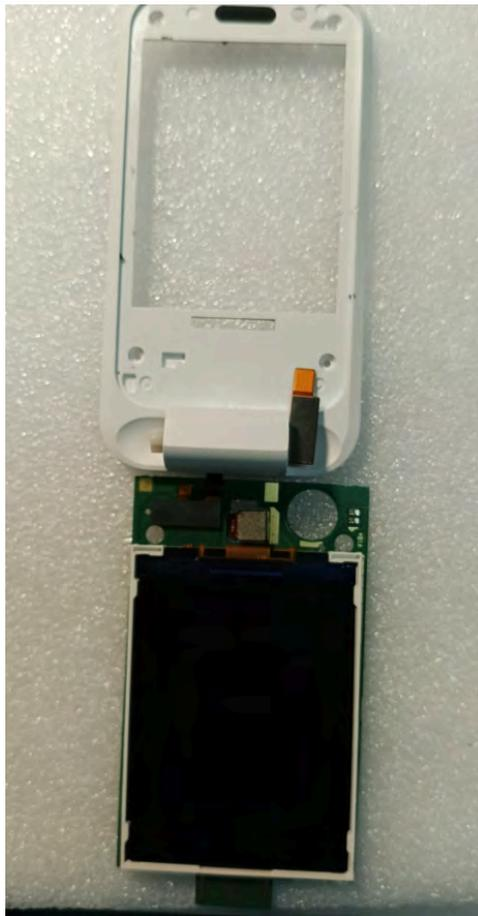
2. Disconnect the **FPC\_LINK\_SF28A\_GF28A1\_6L\_HOLE\_V01A** using **Tweezers**.
