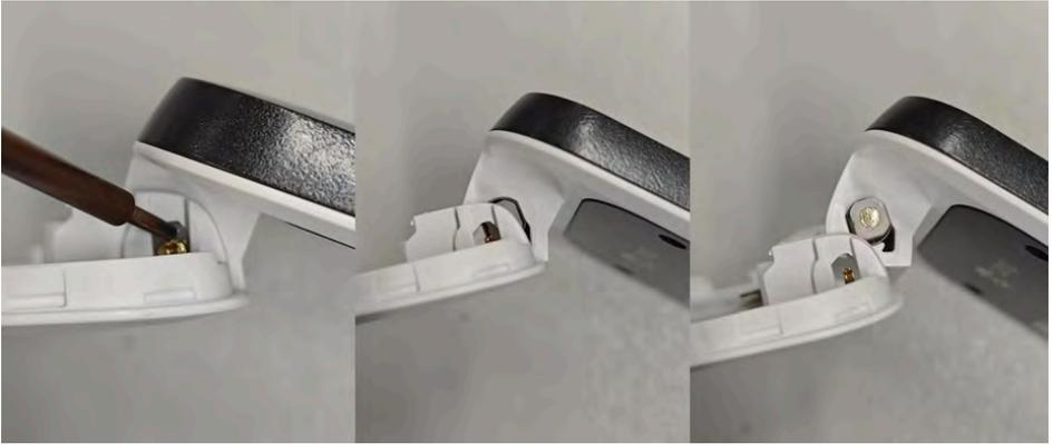
2. Separate the **Clamshell assembly** and the **C-cover**.
