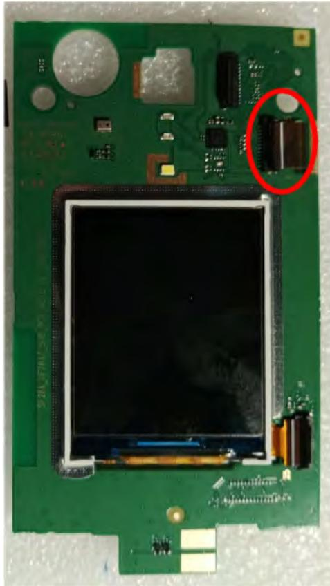
2. Disconnect the flex cable and feed it through the opening to the other side.
