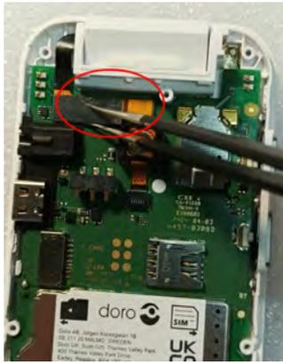
2. Grip the edge of the **PCBA assembly HW1011** and lift it gently.
