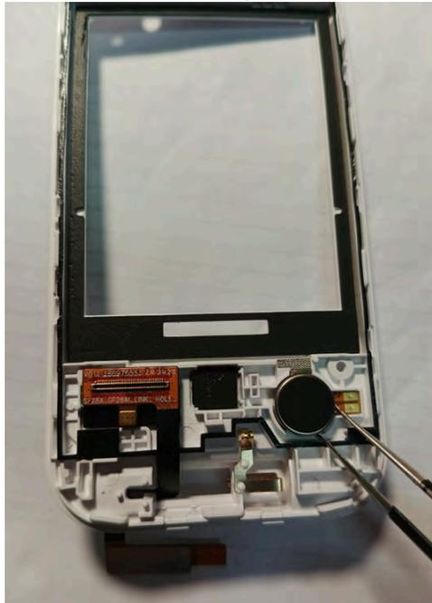
3. Remove the **Main FPC** from the **Assembly up clamshell**.
