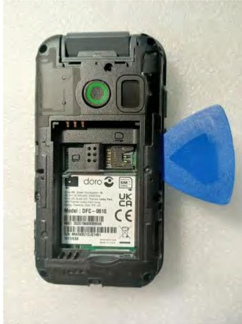
3. Remove the Lower housing assembly .
