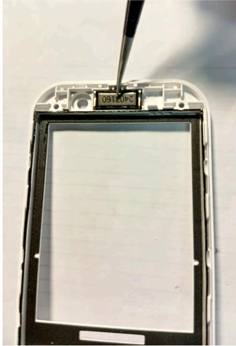
2. Remove the **Motor** from the **Assembly up clamshell**.
