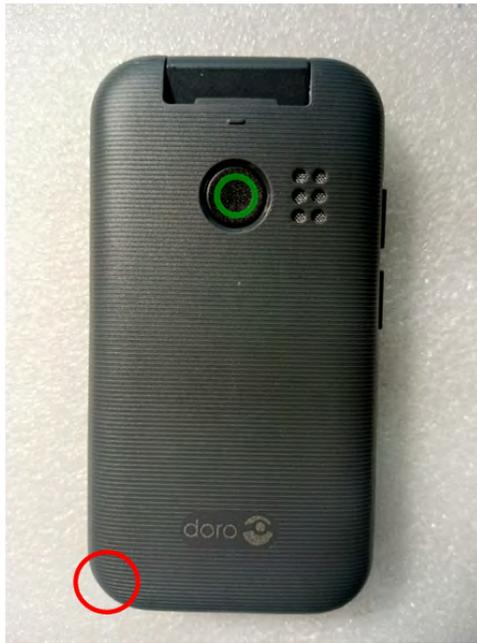
3. Insert a **Plectrum** into the notch and gently slide it along the edges to lift the **Battery cover**.
