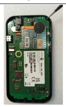
2. Lift the Assembly PCBA HW3011 from the Assembly Upper Housing.
