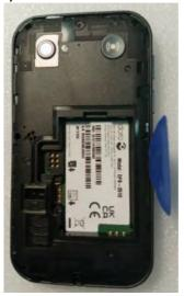
3. Remove the Assembly Lower Housing.
