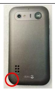
3. Insert a **Plectrum** into the notch and gently slide it along the edges to lift the **Battery Cover**.
