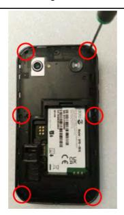
2. Insert the **Plectrum** at the bottom of the device and gently pry open the **Assembly Lower Housing**. Start at the bottom, continue along the sides, and work your way around.
