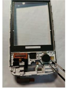
3. Remove the Main FPC from the Assembly clamshell up.
