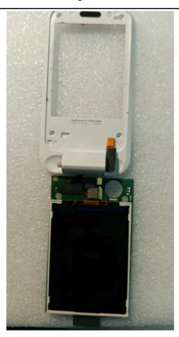
2. Disconnect the FPC LINK SF28A GF28A1 6L HOLE V01A using Tweezers.
