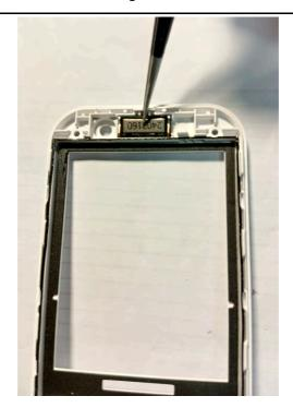
2. Remove the **Motor** from the **Assembly clamshell up**.
