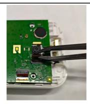
3. Lift the Camera using Tweezers.
