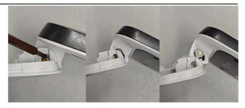
2. Separate the Assembly clamshell and the C cabinet.
