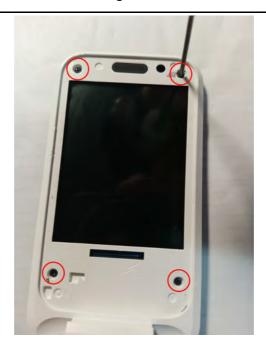
3. Carefully separate the **Assembly clamshell up** from the **Assembly clamshell** along the edge with a **Plectrum**.
