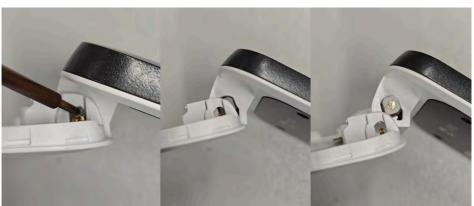
2. Separate the **Assembly clamshell** and the **C cabinet**.
