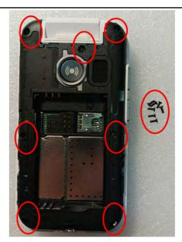
2. Insert the **Plectrum** at the bottom of the device and gently pry open the **Assembly lower housing**. Start at the bottom, continue along the sides, and work your way around.
