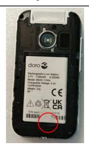
2. Push the Battery LEVA DBAE-1150A outward, then lift it out.
