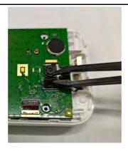
3. Lift the Camera using Tweezers.
