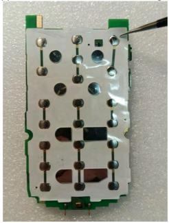
2. Pull the **Dome foil** carefully downwards until it is fully removed.
