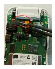
2. Grip the edge of the Assembly PCBA HW3011 and lift it gently.
