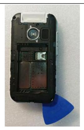
3. Remove the **Assembly lower housing**.
