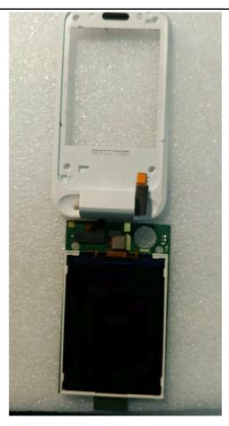
2. Disconnect the **FPC\_LINK\_SF28A\_GF28A1\_6L\_HOLE\_V01A** using **Tweezers**.
