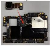
4. Position the PCBA ASSY in the Front housing ASSY and make sure to align it with the screw holes. Fasten the PCBA ASSY with the Screw3 PCBA.
