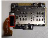
2. Position the **SIM PCB** and align its screw holes with the screw holes on the **Front housing ASSY**.
