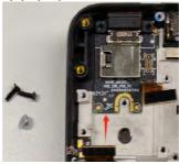
3. Carefully wiggle and pull the **USB PCB** to remove it.
