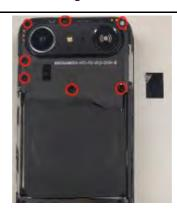
2. Use a Prying lever or a Plectrum to pry off the Rear housing ASSY.
