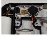
5. Insert the **Prying lever** into the groove next to the **Speaker** and gently pry it up.
