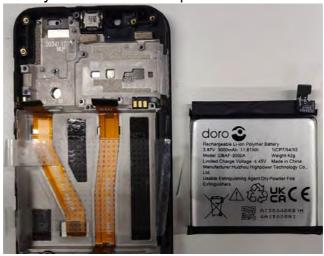
5. Position the replacement **Battery** in the battery compartment of the device.
