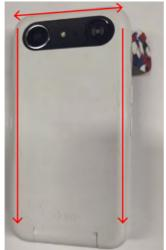
3. Once the top and side edges are loosened, firmly push the **Battery cover ASSY** toward the bottom of the device.
