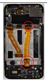
3. Position the **RF cable** cable in the **Front housing ASSY** and connect it to the ports on the **ANT PCB** and the PCBA according to the image.
