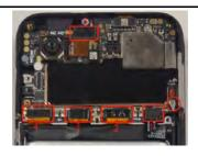
2. Remove the Screw3 PCBA.
