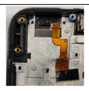
2. Lift off the USB Light sensor FPC.
