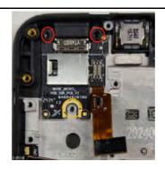
Connect the USB Light sensor FPC in the USB PCB on one end, and let the other hand be loose (until the PCBA ASSY is installed at a later stage).
