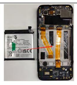
6. Connect the **Battery** to the designated connector (marked red) on the **PCBA ASSY**.
