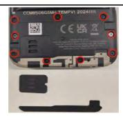
2. Lift off the Speaker bracket ASSY from the device.
