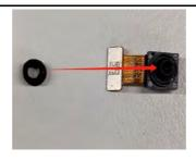
2. Assemble the Front camera 5M with the Rubber sleeve front camera in the Front housing ASSY.
