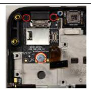
2. Use Tweezers to carefully pry up one end of the USB PCB.
