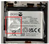
2. Firmly pull the remaining plastic strip to lift the **Battery** out of the battery compartment.
