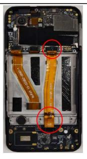
3. Position the **RF cable** cable in the **Front housing ASSY** and connect it to the ports on the **ANT PCB** and the PCBA according to the image.
