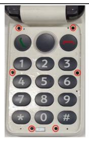
2. Insert the **Pick** between the **Hinge Flip bottom ASSY** and the **Flip decorative part** to pry up the **Flip decorative part**.
