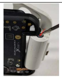
6. The **Front housing ASSY** and the **Hinge Flip bottom ASSY** should be perfectly aligned according to the image.
