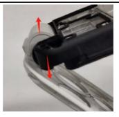
3. Separate the Front housing ASSY and the Hinge Flip bottom ASSY.
