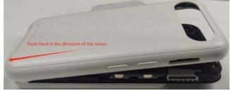
4. Once fully loosened, carefully lift off the **Battery cover ASSY**.
