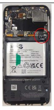
2. Locate the center plastic strip on the protective film. This is the tab used for **Battery** removal.
