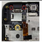
Connect the USB Light sensor FPC in the USB PCB on one end, and let the other hand be loose (until the PCBA ASSY is installed at a later stage).
