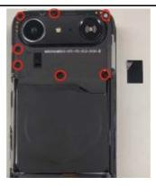
2. Use a **Prying lever** or a **Pick** to pry off the **Rear housing ASSY**. **Note!**
