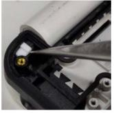
6. Disconnect and remove the Antenna board FPC.
