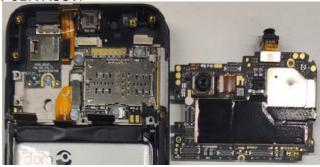
4. Locate and remove the **Front camera 5M** and the **Rear main camera 13M**.
