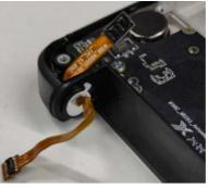
4. Assemble the Sealing silicone B hinge in the other hole on the .
