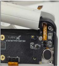
5. To insert the **Hinge** pin on the other side of the **Front housing ASSY** and firmly pushthe **Hinge Flip bottom ASSY** in place using a **Prying lever** or **Tweezers**.
