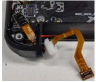
3. Fixate the **Hinge FPC** by fitting the **Sealing silicone A hinge** in the hole on the .
