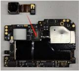
4. Position the **PCBA ASSY** in the and make sure to align it with the screw holes. Fasten the **PCBA ASSY** with the **Screw3 PCBA**.
