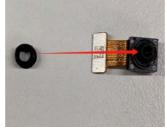
2. Assemble the **Front camera 5M** with the **Rubber sleeve front camera** in the .
