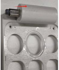
3. The metal shell on the **Hinge** must be fully inserted into the hole of the **Hinge Flip bottom ASSY** according to the image.
