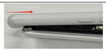
2. Press the rest of the Battery cover ASSY into place.
