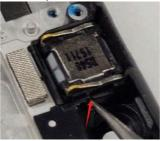
2. Use a Prying lever to pry up the Power key FPC.
