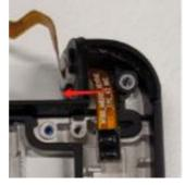
2. Separate the the Sealing silicone A hinge from the Hinge FPC.
