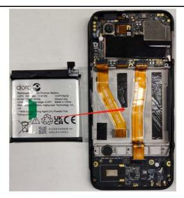
6. Connect the Battery to the designated connector (marked red) on the .
