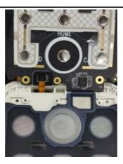
3. Assemble the **Sealing silicone B hinge** over. to the designated connector (marked red) on the **PCBA ASSY**.
