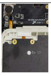
4. Fasten the Key PCB ASSY with the Screw4 flip top bottom cover.
