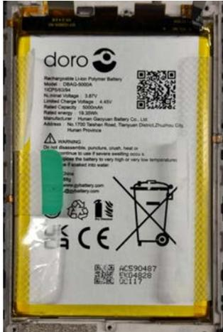
2. Firmly pull the remaining plastic strip to lift the **Battery** out of the battery compartment.
