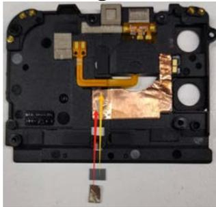
4. Glue the **NFC antenna Charging coil** to the **Rear housing ASSY**.
