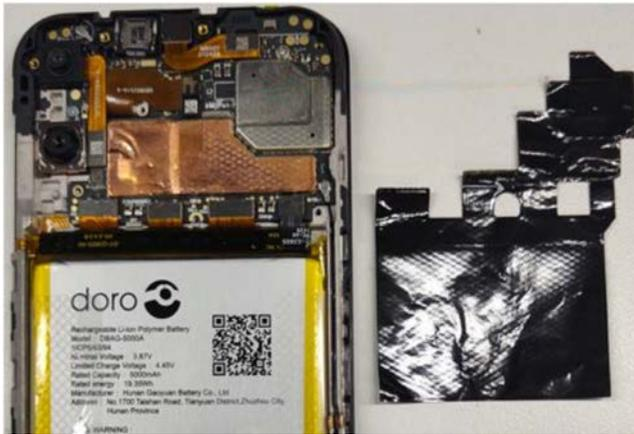
2. Disconnect the **Battery** connector.
