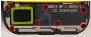
2. Remove the **Antenna bracket ASSY**.
