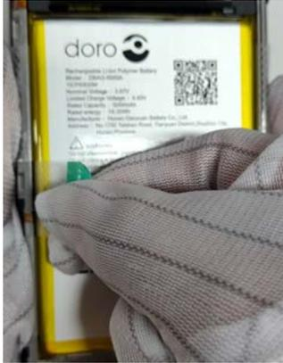
4. Lift off the **Battery** that needs to be replaced.
