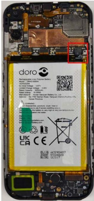
2. Locate the remaining plastic strip on the protective film. This is the tab used for **Battery** removal.
