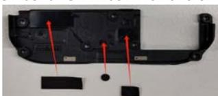
2. Position the **Antenna bracket ASSY** on the device and make sure to align the screw holes.
