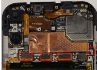
4. Disconnect the **Front camera 5M** and the **Wide angle camera 5M** connectors.
