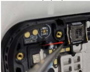
4. Use a **Prying lever** or **Tweezers** to remove the **Pilot lamp PCB**.
