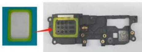
2. Glue the **Motor conductive cloth** in positions according to the images.
