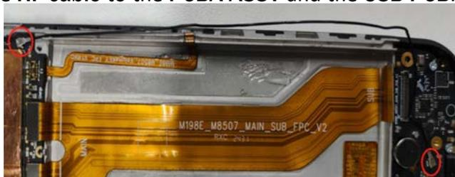
2. Arrange the **RF cable** according to the image.
