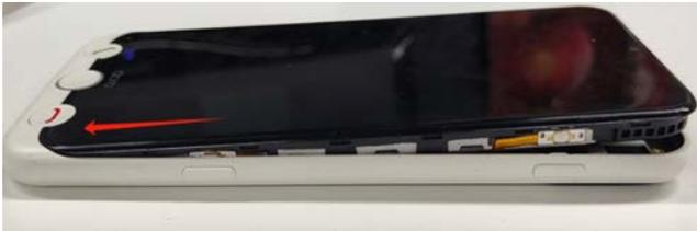
3. Press the rest of the **Battery Cover ASSY** into place.
