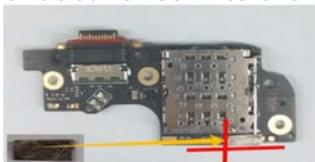
2. Position the **USB PCB** on the **Speaker ASSY** and make sure to align the screw holes.
