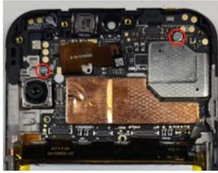
2. Disconnect the **Pilot lamp board RF cable**.
