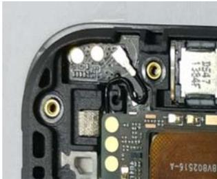
4. Fasten the **PCBA ASSY** with the **Screw2 lock board**.
