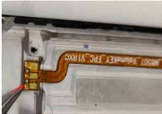
6. Use **Tweezers** to remove the **Power Camera button FPC**.
