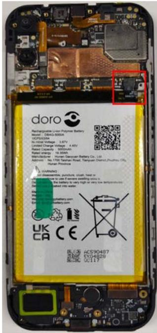
3. Glue the Graphite sheet to the PCB ASSY.
