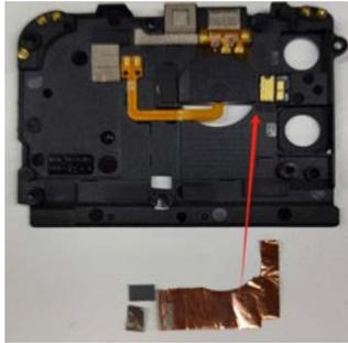
3. Glue the **Receiver ground conductive foam** and the **Flash board cooling silicone** onto the **Rear housing ASSY**.
