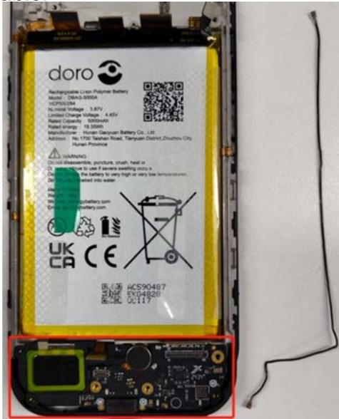
3. Lift off the **USB PCB** (marked red).
