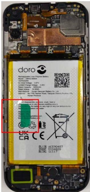
3. Firmly pull the remaining plastic strip to lift the **Battery** out of the battery compartment.
