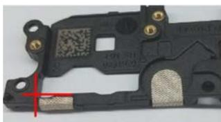
3. Align the **Front key FPC** to the **Speaker ASSY** according to the image and use glue to fasten it.
