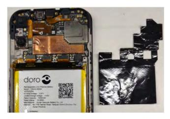
2. Disconnect the **Battery** connector.
