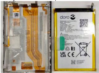
5. Position the replacement **Battery** in the battery compartment of the device.
