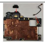
2. Position the PCBA ASSY in the Front housing ASSY.
