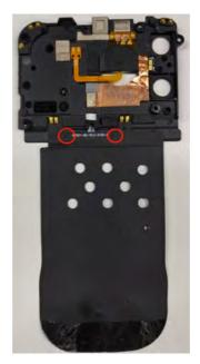
5. Position the **Rear housing ASSY** onto the device and make sure to align the screw holes.
