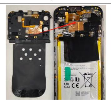
6. Fasten the Rear housing ASSY with the Screw1 lock case.
