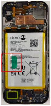
3. Firmly pull the remaining plastic strip to lift the **Battery** out of the battery compartment.
