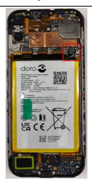
2. Locate the remaining plastic strip on the protective film. This is the tab used for **Battery** removal.
