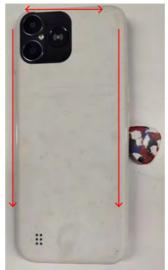
3. Once the top and side edges are loosened, firmly push the **Battery Cover ASSY** toward the bottom of the device.
