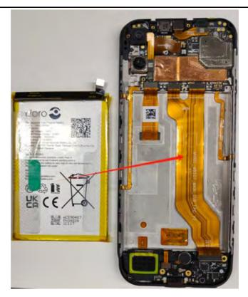
6. Connect the **Battery** to the designated connector (marked red) on the **PCBA ASSY**.
