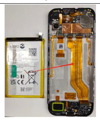
2. Connect the **Battery FPC** to the designated connector (marked red) on the **PCBA ASSY**.
