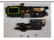
6. Remove the Small board conductive foam from the Speaker ASSY.
