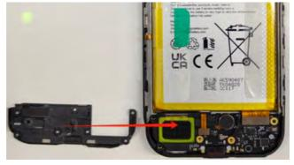
3. Fasten the Antenna bracket ASSY with the Screw1 lock case.
