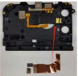
3. Glue the Receiver ground conductive foam and the Flash board cooling silicone onto the Rear housing ASSY.
