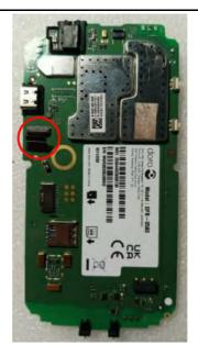
2. Place the LCD 2.4 on the PCBA Assembly HW1011. Align it using the locator lines on the PCBA Assembly HW1011.
