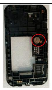
2. Place the **Speaker** into its slot in the **Assembly Lower housing** using **Tweezers**.
