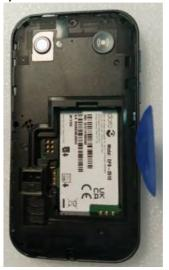
3. Remove the Assembly Lower housing.
