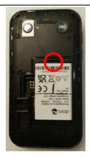
2. Push the Battery LEVA DBAE-1150A outward, then lift it out.
