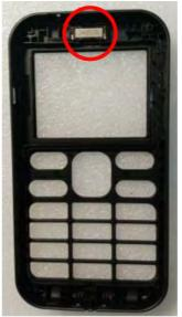
3. Pry the Receiver loose carefully and remove it.
