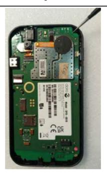
2. Lift the PCBA Assembly HW1011 from the Upper housing assembly.
