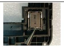
2. Remove the **Motor** from the **Assembly Lower housing** by using **Tweezers**.
