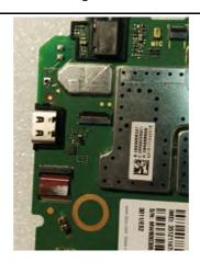
4. Close the ZIF connector to secure the cable.
