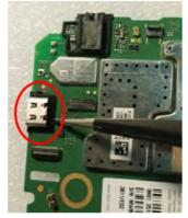
2. Grip the **Sealing rubber 3.5mm jack** with **Tweezers** and lift it from its position.
