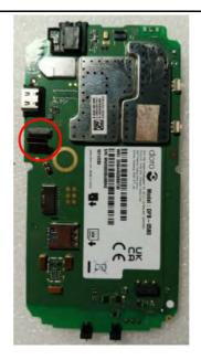
2. Place the new LCD 2.4 onto the PCBA Assembly HW1011.
