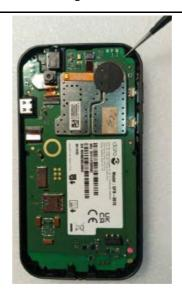
2. Make sure the **Assembly PCBA HW3011** sits evenly and is properly aligned with the frame.
