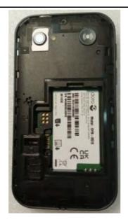
3. Insert and tighten the six (6) screws to secure the **Assembly Lower Housing**.
