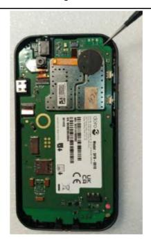
2. Lift the Assembly PCBA HW3011 from the Assembly Upper Housing.
