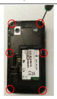
2. Insert the **Prying lever** at the bottom of the device and gently pry open the **Assembly Lower Housing**. Start at the bottom, continue along the sides, and work your way around.
