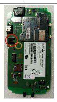
2. Place the new LCD 2.4 onto the Assembly PCBA HW3011.
