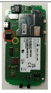
2. Place the LCD 2.4 on the PCBA Assembly HW2011. Align it using the locator lines on the PCBA Assembly HW2011.
