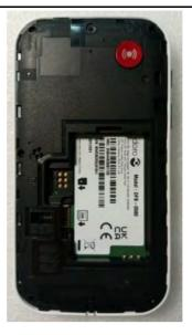
3. Insert and tighten the six (6) screws to secure the **Lower housing assembly**.
