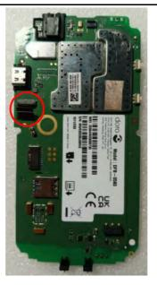
2. Place the new LCD 2.4 onto the PCBA Assembly HW2011.
