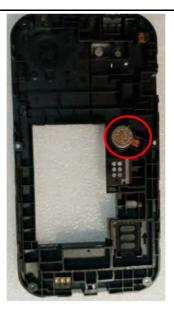
2. Place the **Speaker** into its slot in the **Lower housing assembly** using **Tweezers**.
