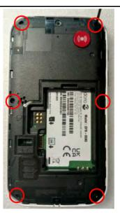
2. Insert the **Prying lever** at the bottom of the device and gently pry open the **Lower housing assembly**. Start at the bottom, continue along the sides, and work your way around.
