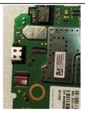
4. Close the ZIF connector to secure the cable.
