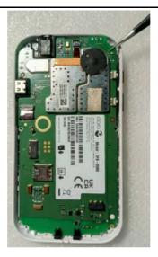
2. Make sure the **PCBA Assembly HW2011** sits evenly and is properly aligned with the frame.
