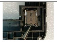
2. Remove the **Motor** from the **Lower housing assembly** by using **Tweezers**.
