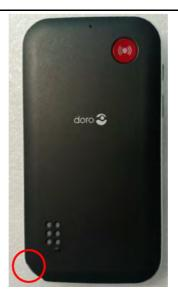
3. Insert a **Prying lever** into the notch and gently slide it along the edges to lift the **Battery Cover**.
