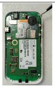
2. Lift the PCBA Assembly HW2011 from the Assembly Upper housing.
