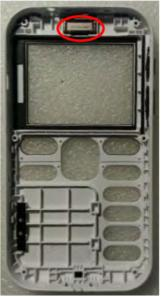
3. Pry the Receiver loose carefully and remove it.
