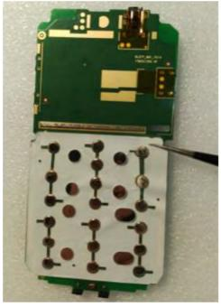
2. Pull the **Dome** carefully downwards until it is fully removed.
