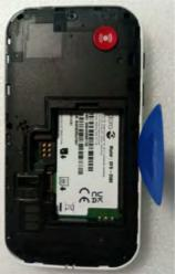
3. Remove the Lower housing assembly.
